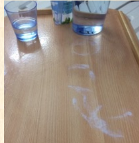
Laminated wood bedside table coated with NanoCote following water spillage
