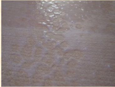
Laminated wood bedside table coated with NanoCote HD-WR (before curing). Close-up view showing uneven distribution after application
