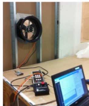
MOCK UP ROOM CREATED TO TEST WALL PENETRATIONS WITH A BLOWER DOOR
