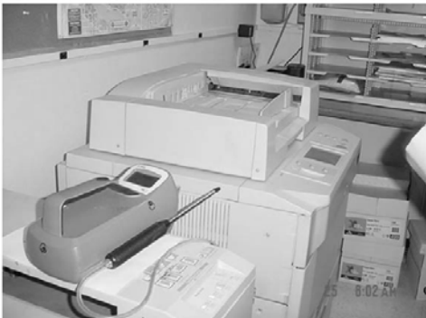
Condensation Particle Counter-0.01 to 1.0 \mu m
